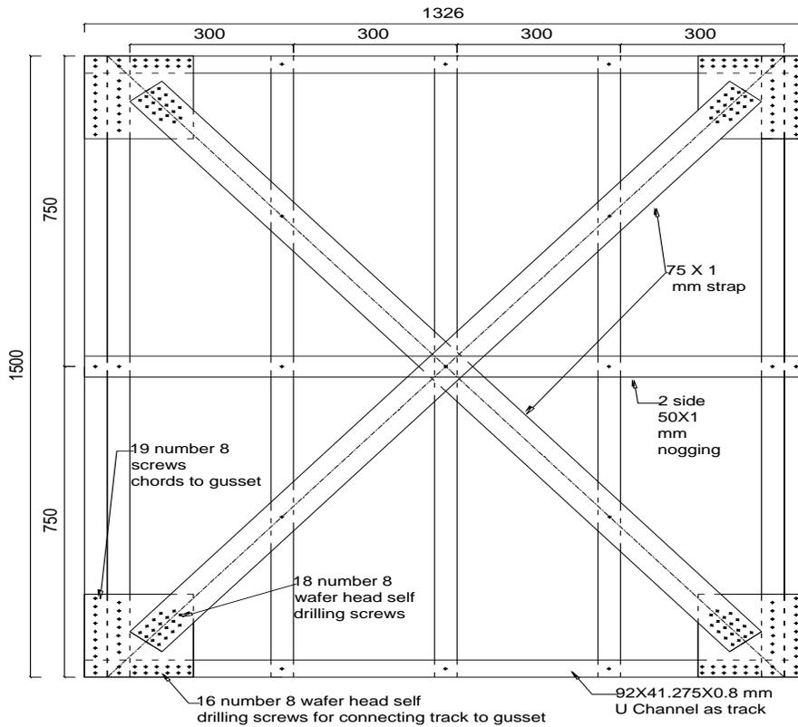
Figure 1. Prototype LSF braced frame
